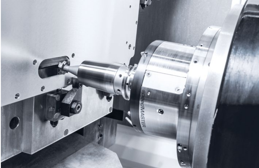
The NHX 8000 machines at PWS are equipped with #40 speedMASTER spindles as a special option.
