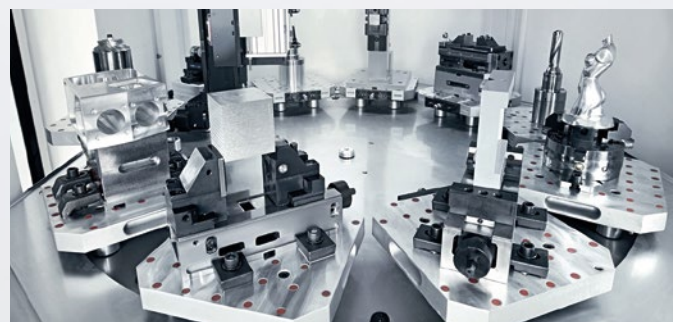
PH 150 – 8-pallet pool; load capacity 551lbs incl. pallet (optional 772lbs)
