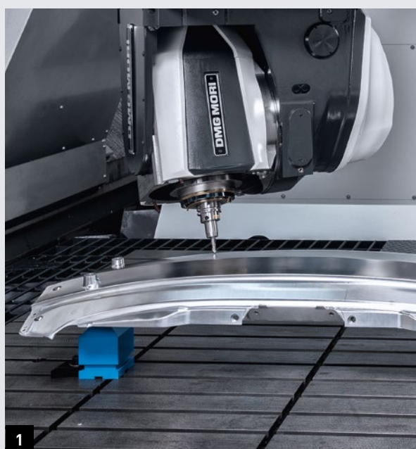
1. 45° or 90° milling head for 5-axis machining at up to 30,000 rpm
